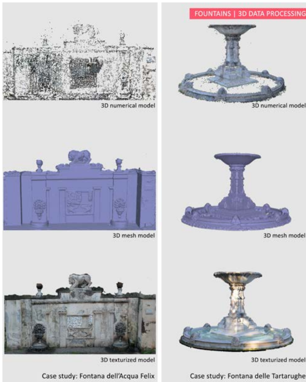
Fig. 5: Definition of 3D model: 3D numerical model, 3D mesh model and 3D texturized model. Case study: Fontana dell'acqua felix and Fontana delle tartarughe
