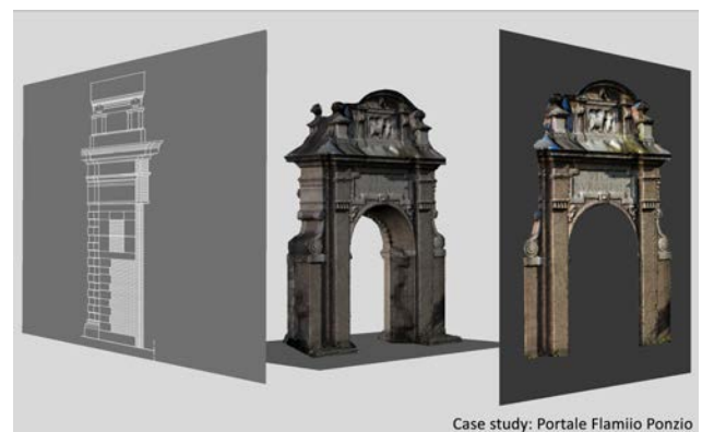
Fig. 7: 2D texturized and architectural model from 3D model. Case study: Portale Flaminio Ponzio
