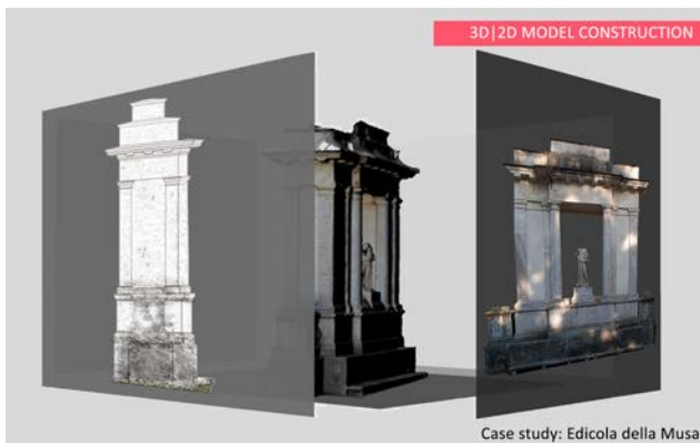
Fig. 6: 2D texturized and architectural model from 3D model. Case study: Edicola della Musa
