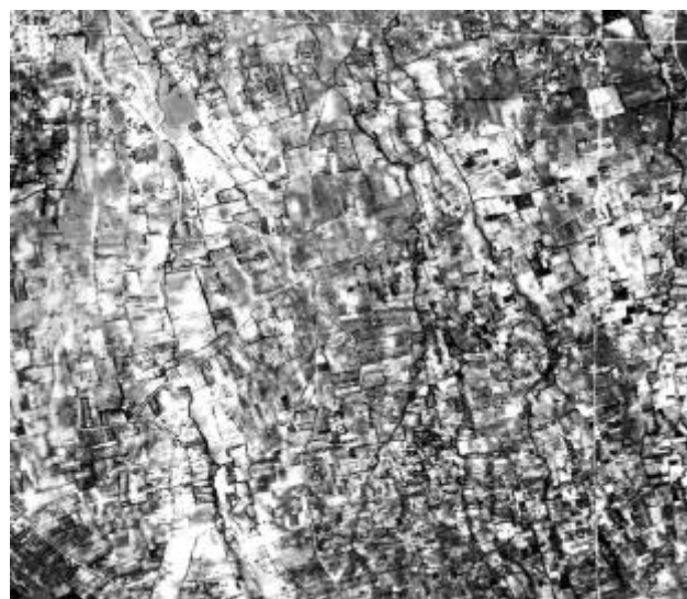
Fig. 2-3: Mosaic (part.). The shadow and damp marks relating to paleo channels of the 'Asso' river network.
